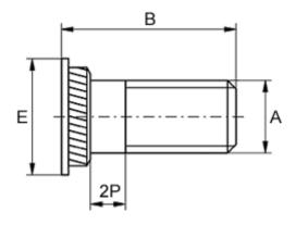
For plate thickness, min = 1.5 Head diameter E = 8 Hole diameter +0.1 = 6.4 Length B = 18 Male thread A = M5x0.8Min distance to edge = 3.3
